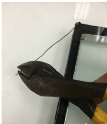
Figure 1: Cutting Tube 1/2" From End
