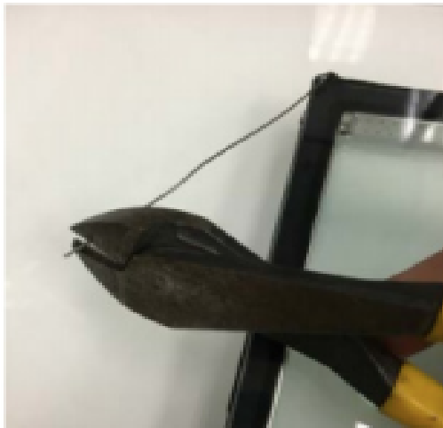
Figure 1: Cutting Tube ½ “ From End
